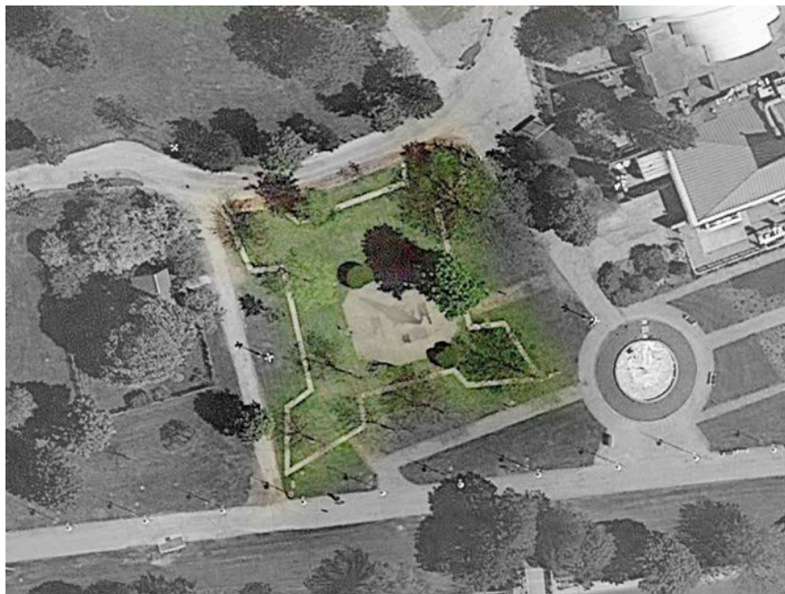
Fig. 14 The image above shows how the star-shaped footprint of Fort Rouille, the historic French fort on the Canadian National Exhibition grounds, was marked with stone setts laid flush into the lawn.
